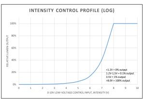
NOTE: The provided information is the typical expected performance of a single luminaire. Additional luminaires on the same 0-10V line may result in different control profiles. Fine tuning of system performance should be completed after installation is complete. To avoid CCT shift between luminaires, care should be taken to minimize voltage drop on the CCT Control line. It is recommended to limit the load on the CCT control circuit to twenty (20) luminaires or less.
