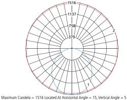
1 - Vertical Plane Through Horizontal Angles (15-195) (Through Max. Cd.)
