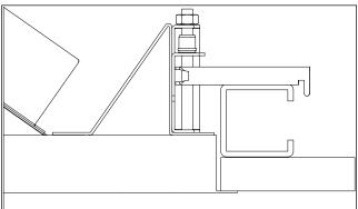
3. Framing around the entire opening is recommended and should start at the rough opening. The minimum thickness of the ceiling material plus the frame material is 1-½ inches. The maximum thickness of the ceiling and framing material is 3 inches. Typically, 1-5/8 Unit trained to frame material because of its strained to start at the rough opening because of its strained to start at the rough opening.
