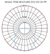
Max Candela = 2816 Located At Horizontal Angle = 15, Vertical Angle = 5 1 - Vertical Plane Through Horizontal Angles (15 - 195) (Through Max. Cd.) 2 - Horizontal Cone Through Vertical Angle (5) (Through Max. Cd.)
