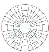
$\label{eq:max-candel} \text{Max Candela} = 1512 \text{ Located At Horizontal Angle} = 0, \text{Vertical Angle} = 0$
