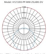
Max Candela = 650 Located At Horizontal Angle = 0, Vertical Angle = 75 1 - Vertical Plane Through Horizontal Angles (0-180) (Through Max. Cd.) 2 - Horizontal Cone Through Vertical Angle (75) (Through Max. Cd.)
