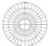
Max Candela = 1266 Located At Horizontal Angle = 0, Vertical Angle = 0
