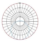
Max Candela = 582 Located At Horizontal Angle = 0, Vertical Angle = 0
