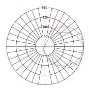
$\mbox{Max Candela} = 560 \mbox{ Located At Horizontal Angle} = 0, \mbox{Vertical Angle} = 80$
