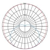
Max Candela = 364 Located At Horizontal Angle = 90, Vertical Angle = 17.5
