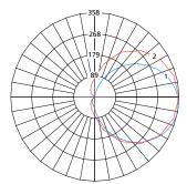
Max Candela = 358 Located At Horizontal Angle = 90, Vertical Angle = 82.5
