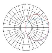
Max Candela = 291 Located At Horizontal Angle = 0, Vertical Angle = 80
