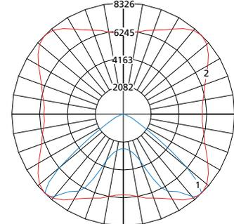
Max Candela = 8326 Located At Horizontal Angle = 45, Vertical Angle = 42.5
