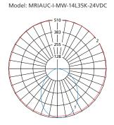
Max Candela = 510 Located At Horizontal Angle = 60, Vertical Angle = 5 1 - Vertical Plane Through Horizontal Angles (60-240) (Through Max. Cd.) 2 - Horizontal Cone Through Vertical Angle (5) (Through Max. Cd.)
