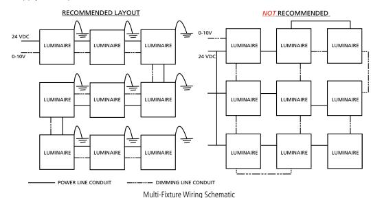
8. Make DC supply and (optional) dimmer control connections within each luminaire.
