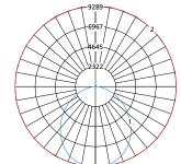
Max Candela = 9289 Located At Horizontal Angle = 0, Vertical Angle = 5
