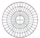
Maximum Candela = 3170 Located At Horizontal Angle = 15, Vertical Angle = 2.5
