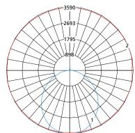
Maximum Candela = 12851 Located At Horizontal Angle = 15, Vertical Angle = 5
