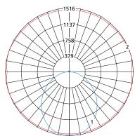
Maximum Candela = 1241 Located At Horizontal Angle = 15, Vertical Angle = 5
