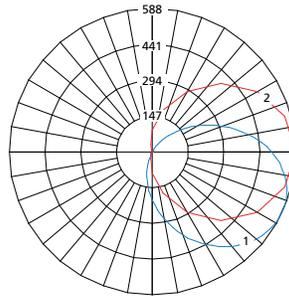
Max Candela = 588 Located At Horizontal Angle = 0, Vertical Angle = 65
