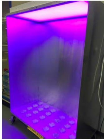
Figure 1. Indigo-Clean™ light fixture and experimental set up for light exposure of bacteria seeded onto agar surfaces.
