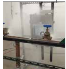
Water Ingress Testing
